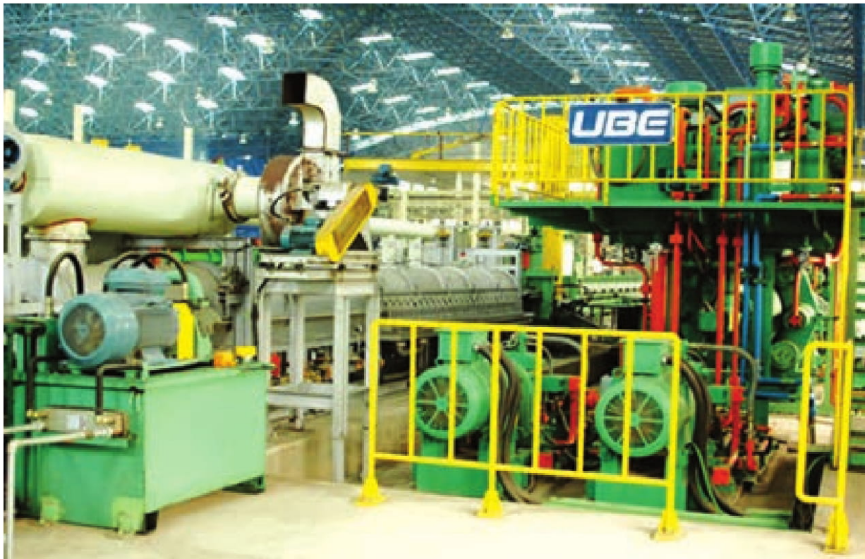
Extrusion production line 1800 ton supplied by UBE - Japan
