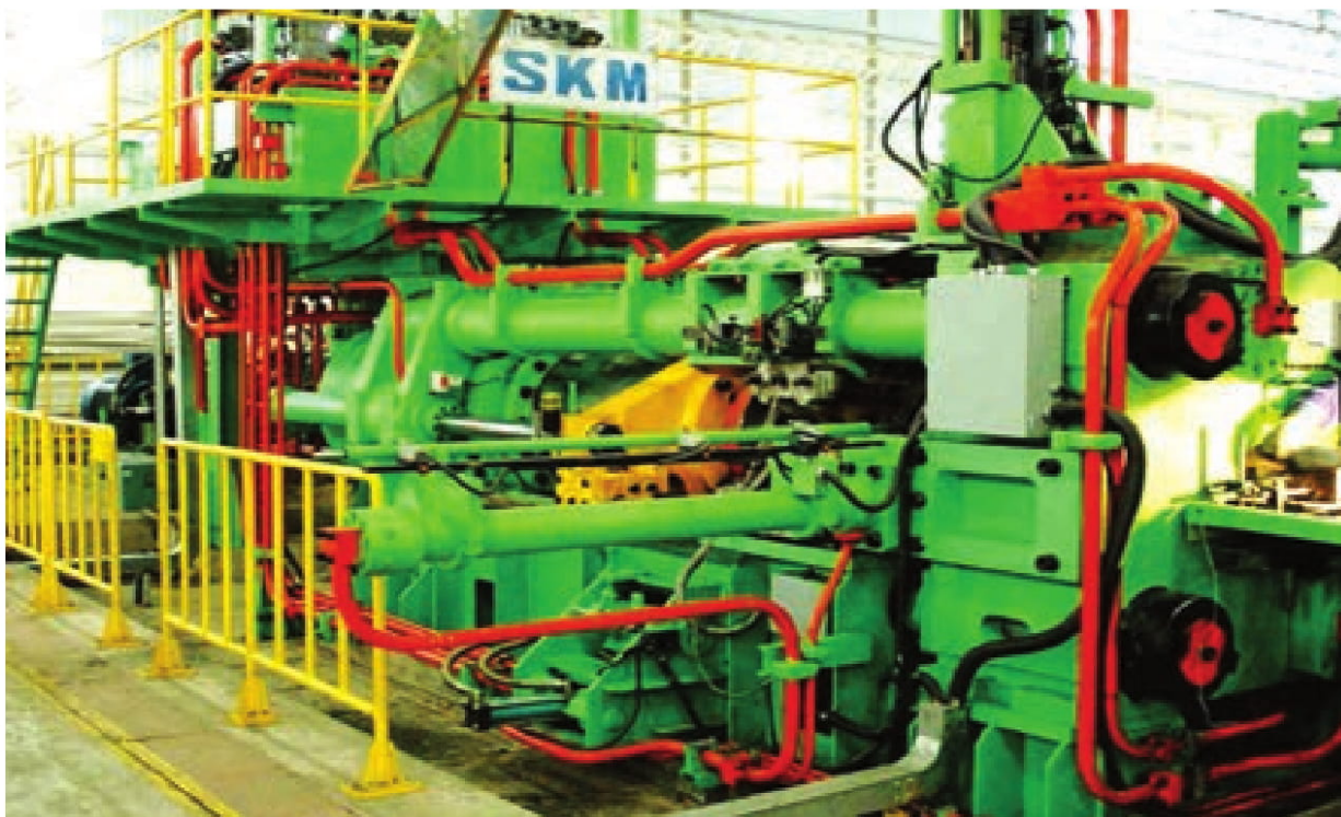
Extrusion production line 1350 ton supplied by Sunkyung - Korea
